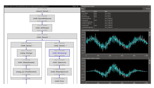
**Figure 3**. Marsyas Inspector displaying a dataflow network, a list of control values and two plots of data at different stages of processing (before and after applying the windowing function).
