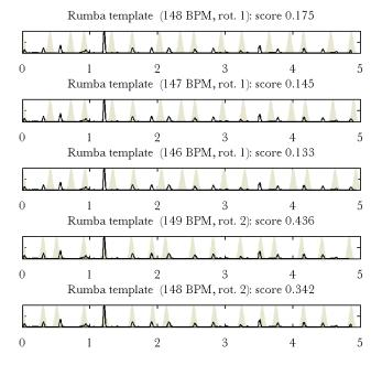
**Figure 4**. Matching different templates (filled grey) to the *CB* recording's energy envelope (black line). The X-axis is time (seconds), with zero the time of the onset under consideration. The score for each template match represents how well that template lines up with the energy envelope.
