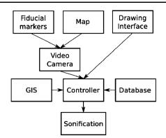
Fig. 2 A flowchart of the system organization of our system. This system has at its core a Controller module that communicates with the phenology and GIS databases as well as the video camera and sonification engine. It generates sonifications by tracking the positions of fiducials on a printed paper map
