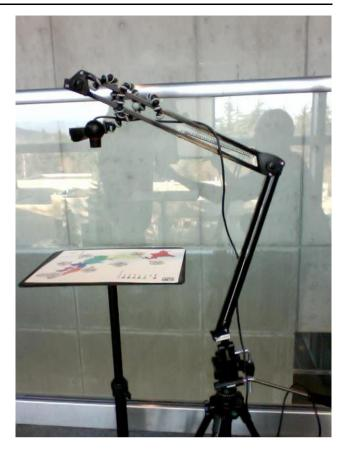
Fig. 3 Shown above is a picture of the fiducial tracking interface. Above the computer monitor is a small consumer grade video camera, which is pointed downwards in order to view the fiducial markers which are placed on a printed paper map
