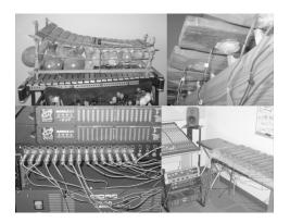
Figure 1: Top left: Gyil on top of vibraphone for showing scale, Top right: piezo sensors under bars, Bottom Left: 2882 input, Bottom Right: overview
