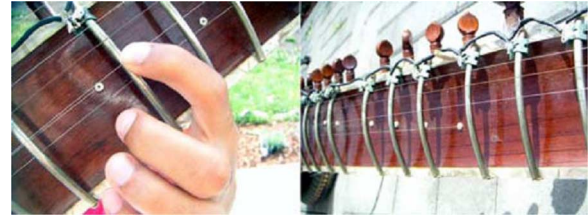
Fig. 3. E-Sitar and thumb sensor.
