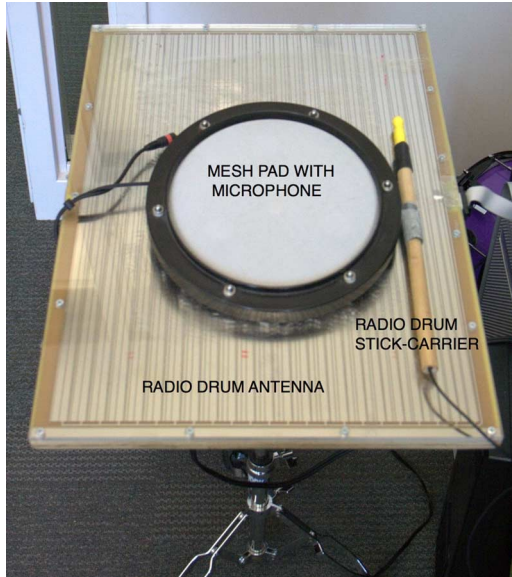
Fig. 5. Drum pad on radio drum surface.
